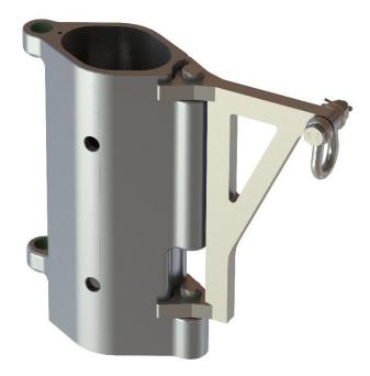
This lifting eye also has a WLL of 500 kg and can be attached in all JibFlex configurations that ends with a 400 mm module. The weight of this lifting eye is 4 kg.
