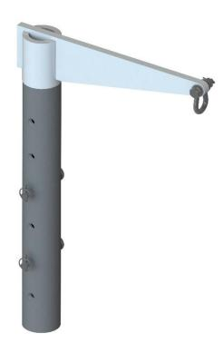
Two locking pins secures it and transfers the forces to the jib arm. The locking pins defines the height of the lifting eye. There are three standard heights of storks with respectively six, seven and eight holes. The weight of the storks are 11.2 kg, 12.2 kg and 13.2 kg respectively.
